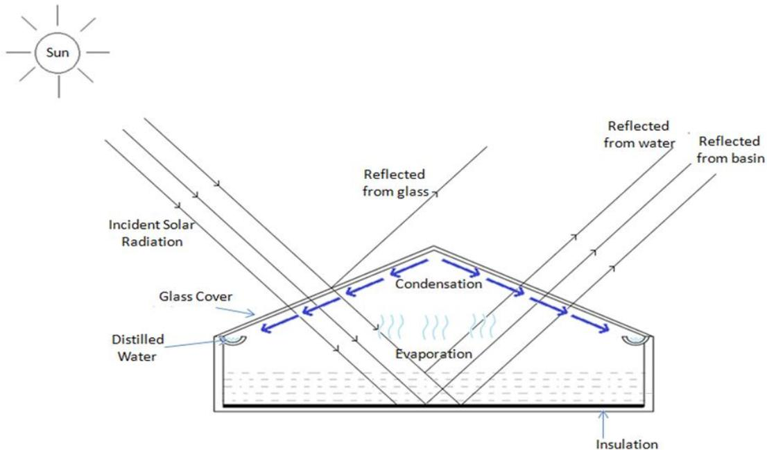
**Fig .1A** Schematic Diagram of Solar Still
