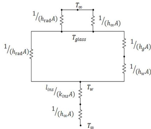
**Fig .3.**Thermal circuit
