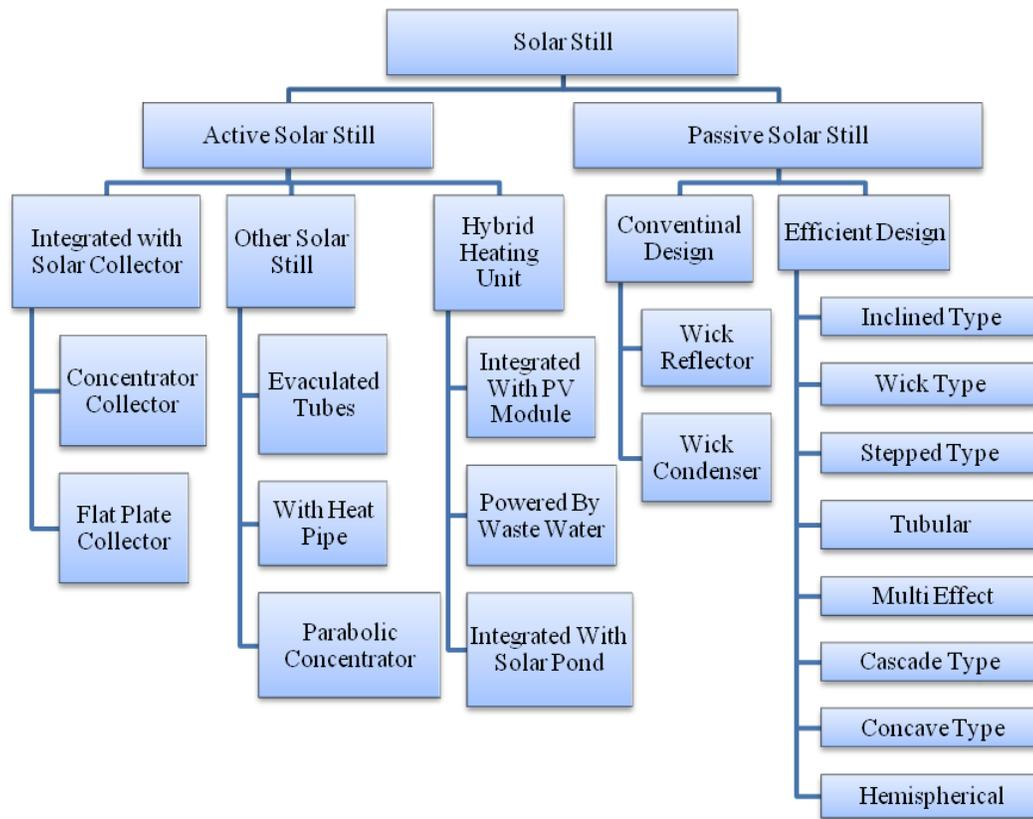
Fig. 2. Classifications of solar still distillation
