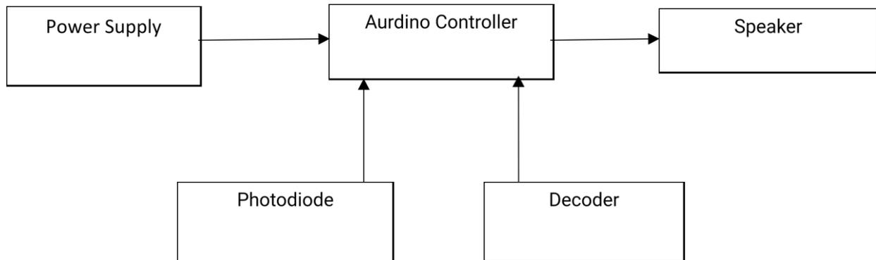
Fig.2. Receiver Part of Indoor Navigation System.
